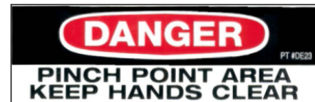
Figure 12: Pinch point decal (DE23) -Located at points where moving parts come close together, mostly on the boom. -Keep clear of pinch points.
