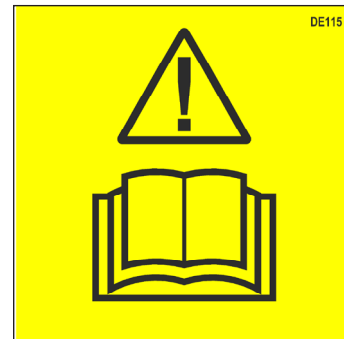
Figure 5: Read Owner's Manual Warning (DE115) -Located at components that require operator adjustment -See Owner's Manual for information on components requiring operator adjustment.
