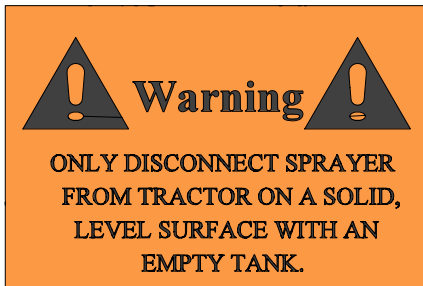
Figure 4: Disconnecting Sprayer (DE136)
