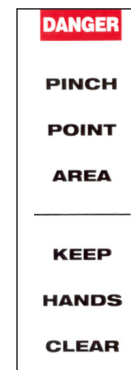
Figure 13: Pinch point decal (DE22) -Located at points where moving parts come close together, mostly on the boom. -Keep clear of pinch points.
