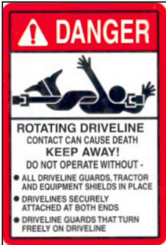
Figure 1: PTO warning decal -Located on the PTO driveline guard.
